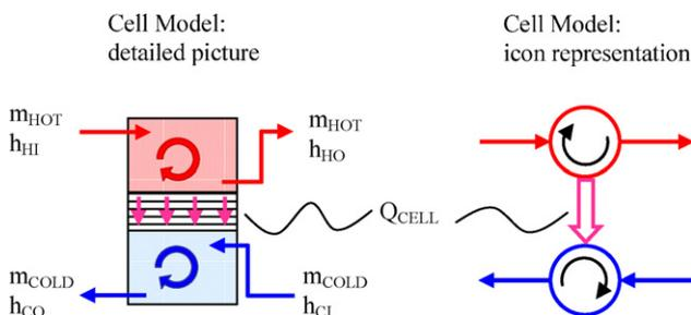
**Fig. 1.** Representation of a modelling cell.
