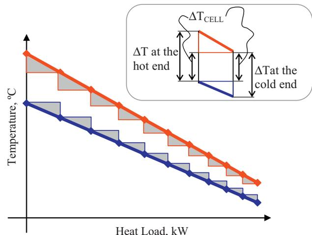
Fig. 3. Driving forces decrease in the cell model.
